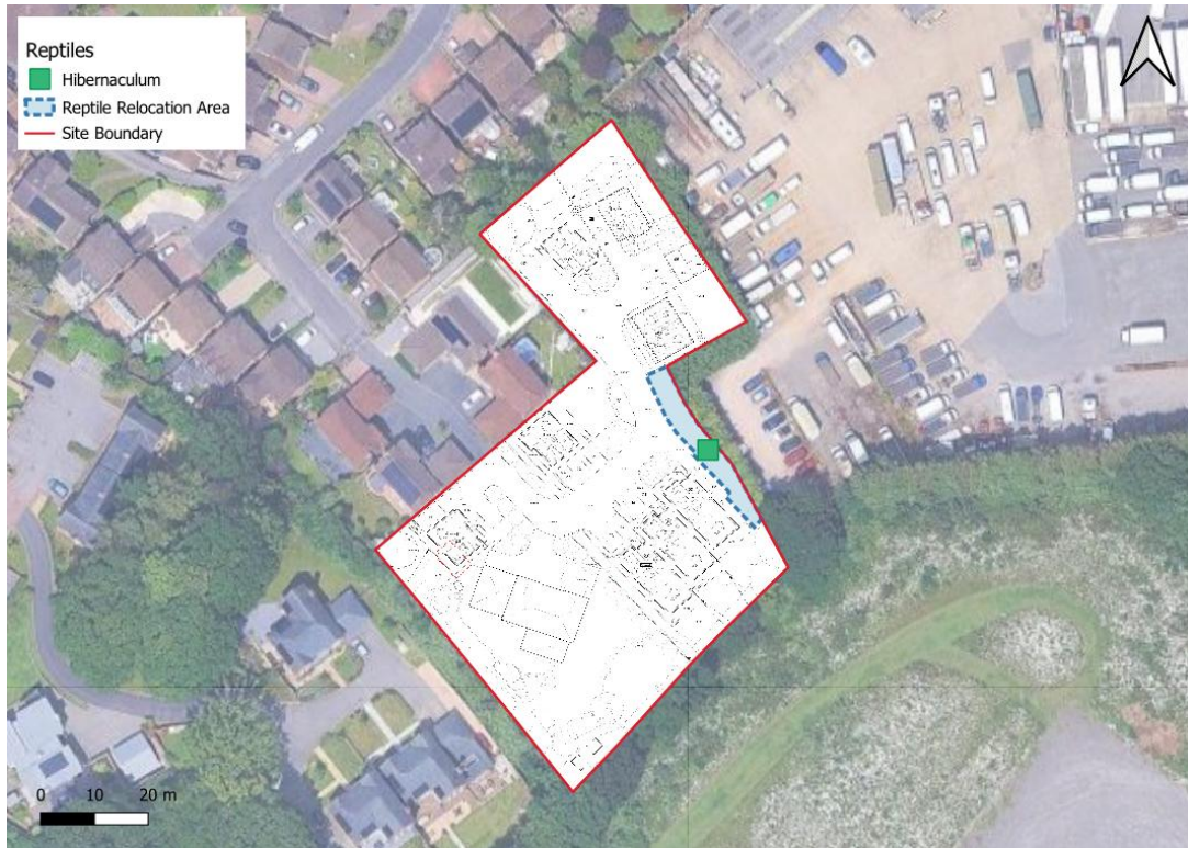
Figure 5. Reptile receptor area (shown in blue) along the eastern boundary of the site, with location of hibernaculum in centre of receptor (green square) and protected during construction by HDPE fencing (blue dotted line).
